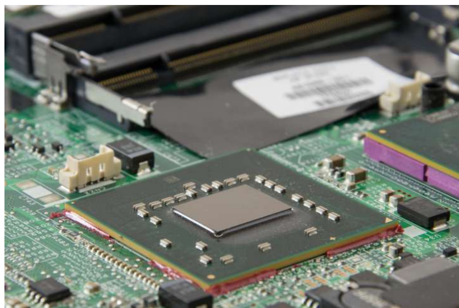
Figure 2.13: A GPU on a PCB board
