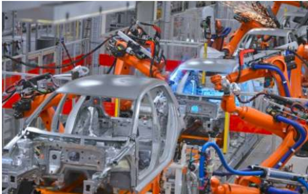
Figure 1.3: Robots welding in an automotive factory
