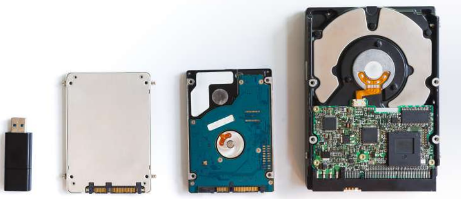
Figure 2.10: Storage devices from left to right: flash drive, SSD, laptop hard drive and internal hard drive
